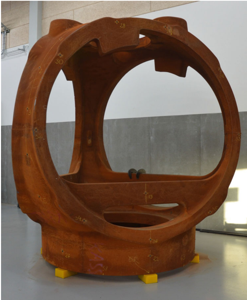
Fig. 8.1 Vestas V112 hub placed on Polyurethane blocks for vibration isolation. The blocks effectively isolates the hub from the surroundings
