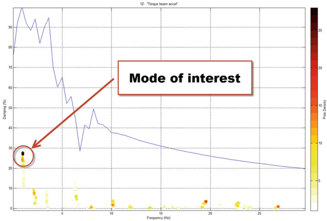
Fig. 30.12 Pole density diagram from LSCE estimates
