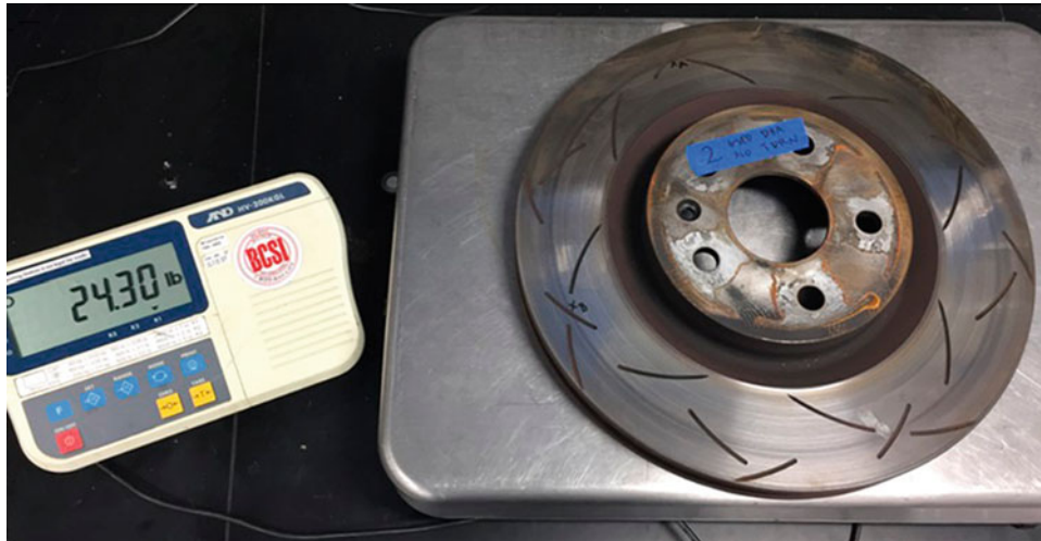
Fig. 13.2 Weight measurement of rotor 2
