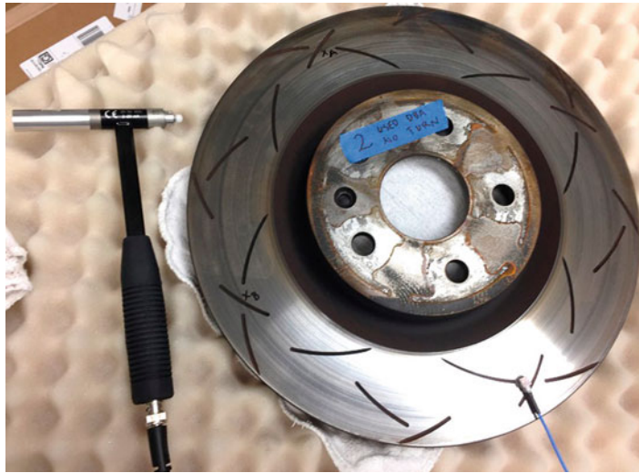
Fig. 13.4 Test set up for Used DBA rotor (#2) showing modal hammer, foam base, accelerometer location, and hammer locations A and B
