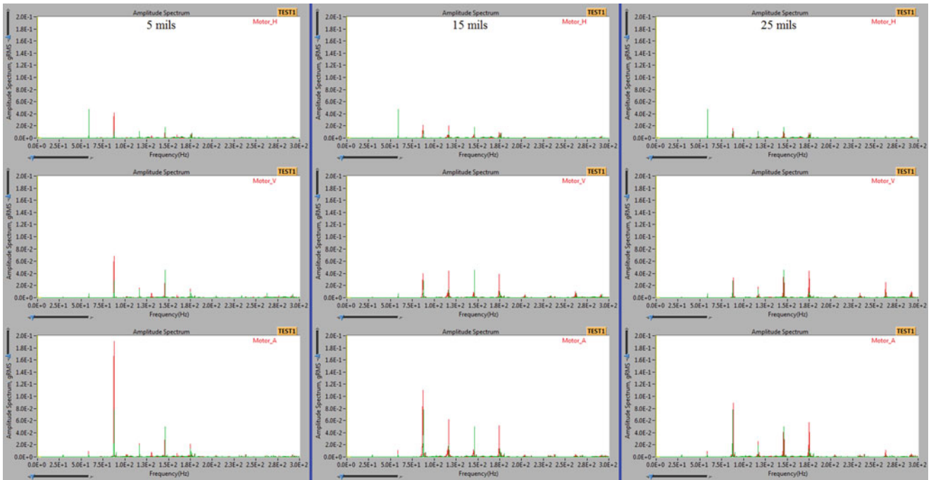
Fig. 20.7 Spectrum of parallel misalignment in red, alignment in green (motor side). Coupling type: spiral, shaft speed: 1750 rpm, shaft diameter: 3/4"
