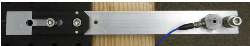
Fig. 16.3 Resonator assembly attached to breadboard
