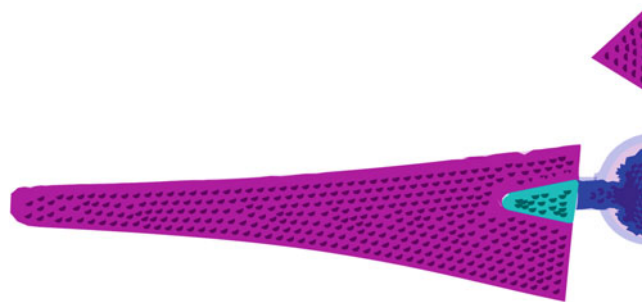
Fig. 13.2 Blade scan points shown on the finite element model
