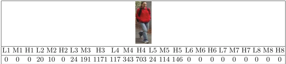
Fig. 5. An example of generated image signature by using FCA approach. On this, 8 dominant colors have been defined by fuzzy system.
