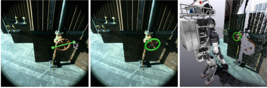
Fig. 6 Fitting the valve affordance. User provides simple annotation in the 2D camera image (left), the fitting algorithm fits a valve affordance, results shown in 2D (middle) and in the 3D view (right)
