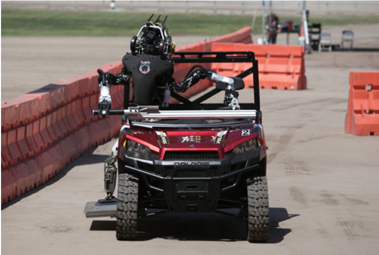
Fig. 9 MIT Atlas robot performing the driving task on Day 1 of the DRC Finals
