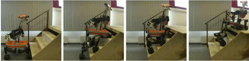
Fig. 25 Momaro climbs stairs, using a specially designed stair gait
