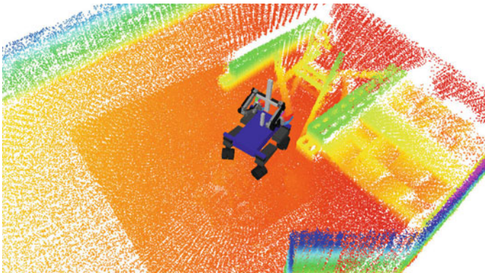
Fig. 15 Point cloud of the egocentric multiresolutional surfel map, as viewed by the robot operator during the debris task of the first DRC competition run. Color encodes height
