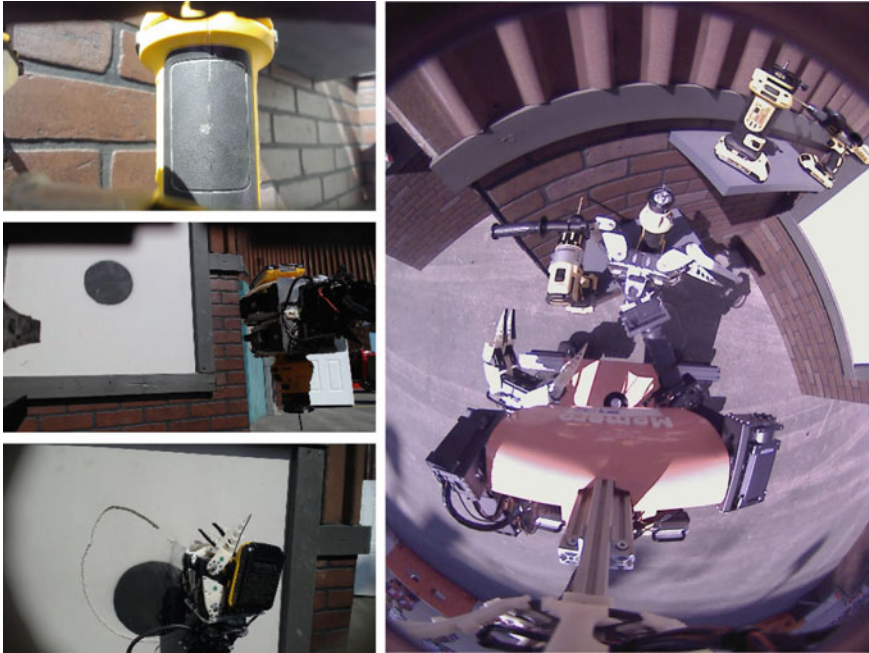
Fig. 23 Top Left: Grasping the cutting tool as seen from the right hand camera. Right: Same scene as seen from the top-down camera. Middle Left: Grasp used to switch on the tool. Bottom Left: Momaro cutting the drywall as seen from a sensor head camera
