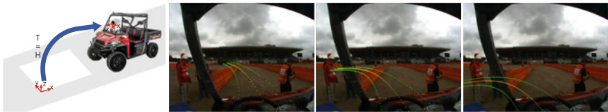
Fig. 34 Concept of predicted driving trajectory projection for manual driving task. Leftmost image depicts the mapping between the ground plane and the camera coordinates to project the trajectory. The other images are examples of predictive driving trajectory projection in the DRC Finals
