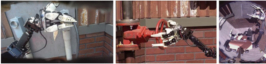
Fig. 22 Left: Inserting the plug as seen from the right hand camera. Middle: Momaro turns the valve. Right: Flipping the switch as seen from the top-down camera
