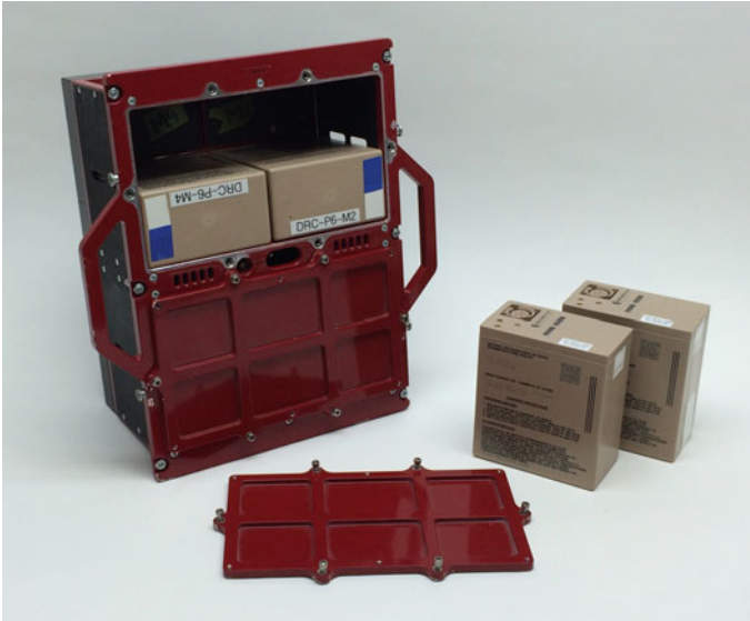
Fig. 17 CHIMP's battery pack and Li-ion battery modules
