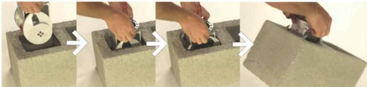
(d) Cam mode: applied one fingertip force during actuation is rated to be 609 N
