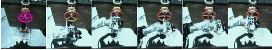
Fig. 20 Robot’s camera view from Valve task. From left to right: Valve Template aligned, Pre-grasp, Grasp, Open affordance 45°, 135°, and 270°
