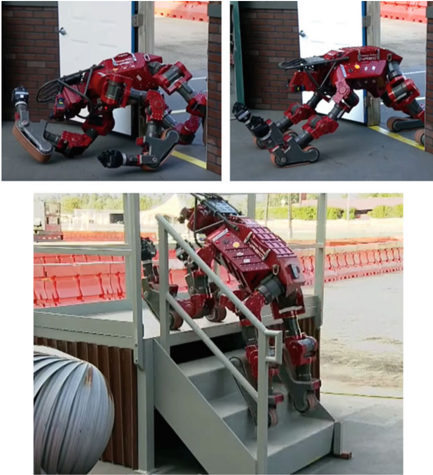
Fig. 8 Team Tartan Rescue taking advantage of their unique robot morphology to recover after falling through the doorway (top) and to climb the stairs using their moveable limbs with embedded wheels and tracks (bottom). Photos from https://www.youtube.com/watch?v=FRkYOFr7yPA (accessed August 2017)
