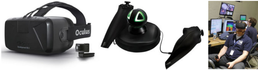
Fig. 17 Immersive telemanipulation. Left: Oculus Rift DK2 HMD. Center: Razer Hydra magnetic trackers. Right: Upper body operator using the HMD and trackers during DRC
