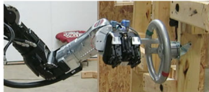
(d) Once the operator confirms, the behavior proceeds to insert the wrist attachment and turn the valve.
