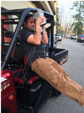
(b) Reacted grasp strength: one fingertip force is rated to be 3kN
