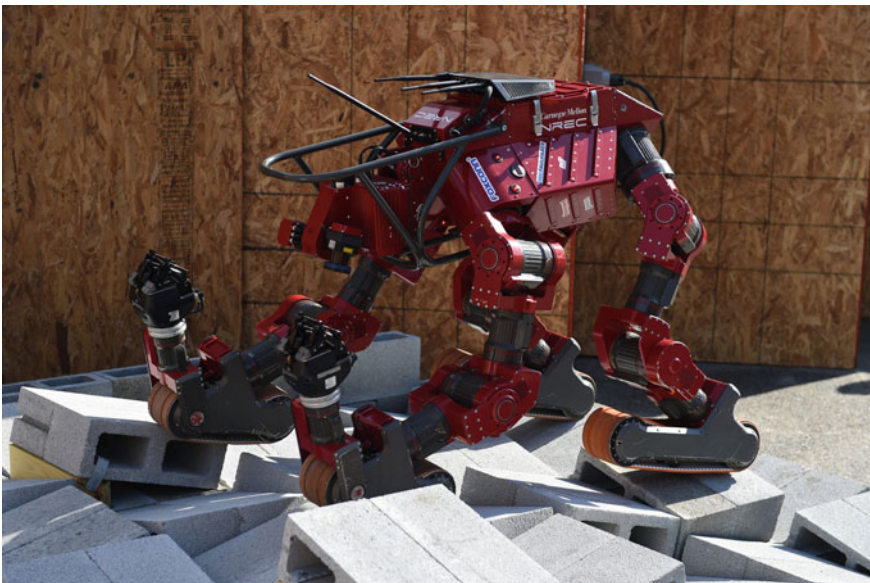
Fig. 4 CHIMP crossing the mobility course at the DRC testbed
