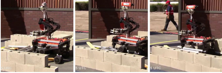
Fig. 24 Momaro pushes through loose debris at the DARPA Robotics Challenge
