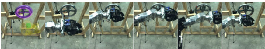
Fig. 24 Robot’s camera view from Valve task. From left to right: Valve Template aligned, Pre-grasp, Grasp, Open affordance 90, 180, and 270°
