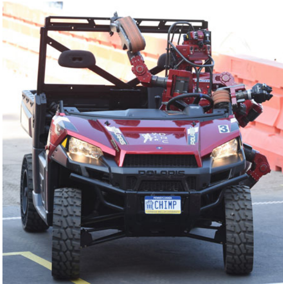
Fig. 2 CHIMP in the polaris vehicle at the DRC finals, controlling the steering wheel with the track belt on the robot’s left arm
