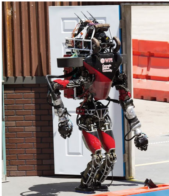
Fig. 1 The ATLAS Unplugged humanoid robot developed by Boston Dynamics
