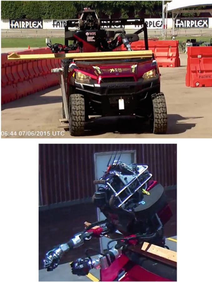
Fig. 19 Driving and egress (getting out of the car) tasks
