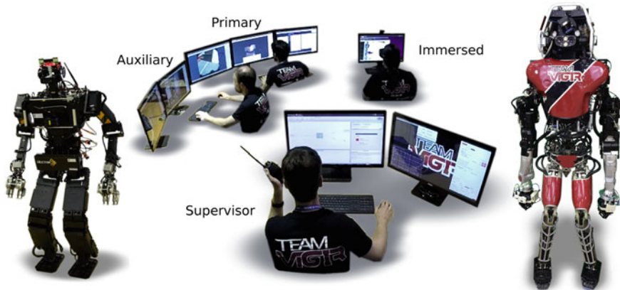
Fig. 1 THORMANG “Johnny” developed by ROBOTIS and used by Team Hector (left), Atlas “Florian” developed by Boston Dynamics Inc. (BDI) (right) and the Operator Control Station (middle) used by Team ViGIR. Both humanoid platforms use the same high-level software to perform remote tasks with human supervision. Operator roles are described in detail on Sect. 3.4
