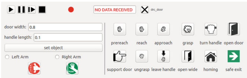
Fig. 23 Door opening task widget. The operator can specify the door data and with which arm the robot should open the door, then the single actions are triggered by associated buttons
