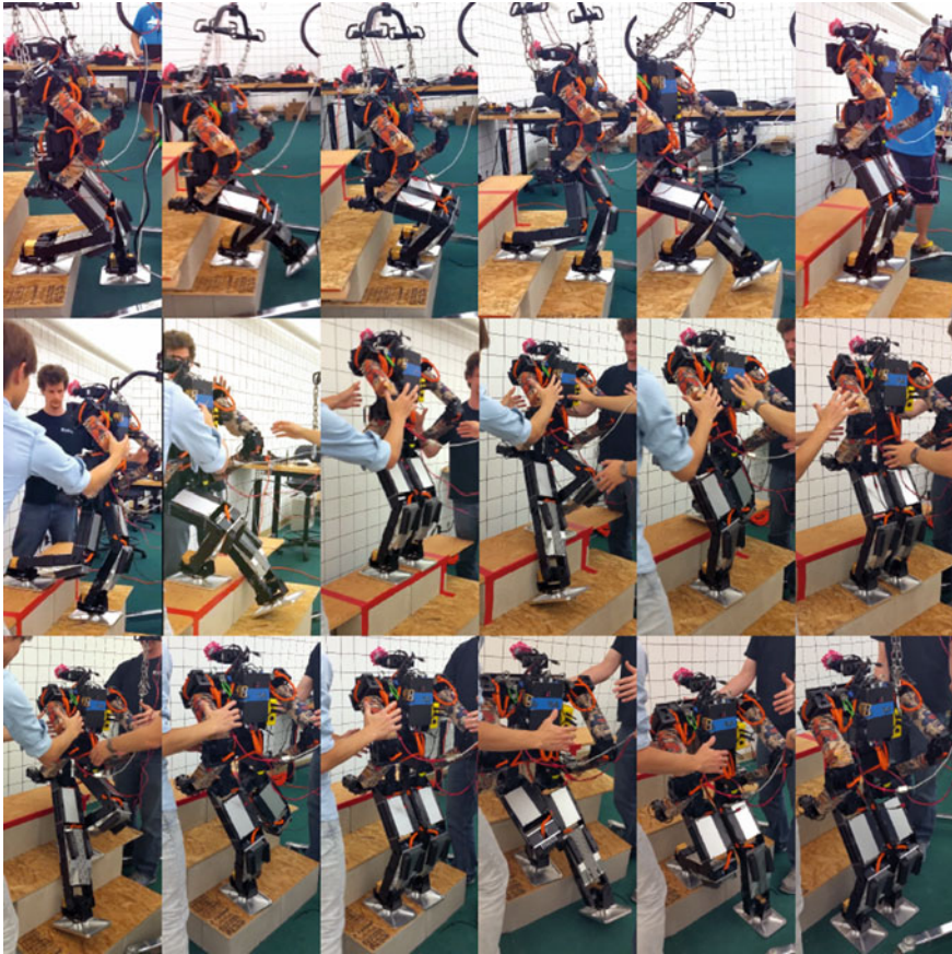
Fig. 27 The THOR-RD robot climbing a set of stairs using the toe and heel lift controller
