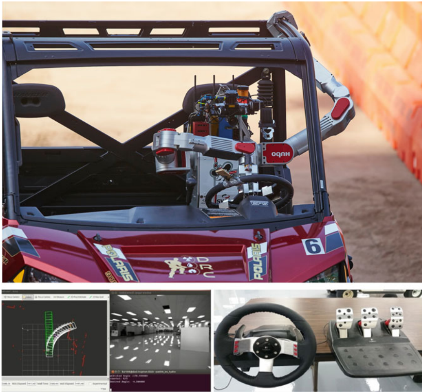
Fig. 11 Team DRC-HUBO at UNLV performing the Vehicle task. Top : The robot operating the car. Photo from http://www.drc-hubo.com/ (accessed August 2017). Bottom : the operator's interaction method for driving the car, showing the car trajectory on the left and the steering wheel and foot pedal input devices on the right. Image from Oh et al. (2017)
