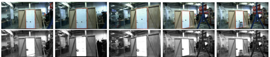
Fig. 14 First row shows detected doors at various perspectives. Second row shows the color based segmentation by searching within the detected door
