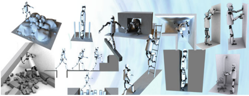
Fig. 22 Some of the mobility tasks that humans excel at due to their morphology and dimensions. Humanoid robots have the potential for achieving human level mobility, including being able to accomplish these mobility tasks, and thus are well suited for operations in complex, cluttered environments found in disaster scenarios as well as every day human environments. Many of these tasks are difficult for wheeled and tracked vehicles that do not have leg-like appendages
