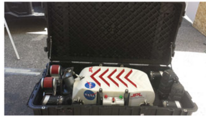
(c) RoboSimian was designed to fit into a standardized military transport case for ease of deployment in a disaster scenario (Pelican, 2016). The interior dimensions of the case are 1.21m (L) X 0.61m (W) X 0.45m (H) .
