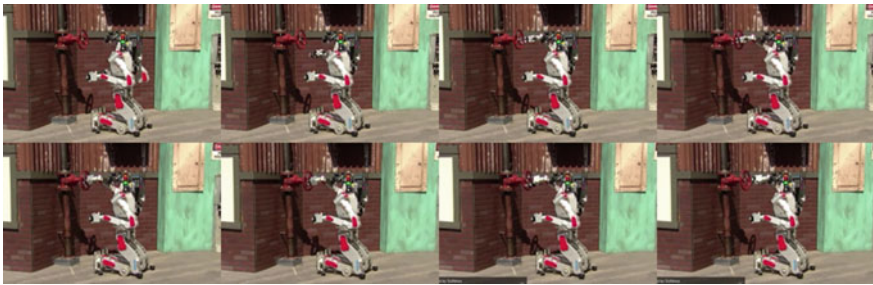
Fig. 26 Valve turning task of DRC-Hubo+ in DRC-Finals (from SciNews)
