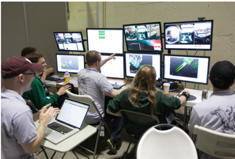
Fig. 5 Team MIT's operator control unit at the DRC Finals. The left most and right most columns of displays are situational awareness monitors with dedicated attendants. The middle four displays belong to the primary operator. Clockwise from top left, they are: process management interface, camera situational awareness, main window with affordance models and teleoperation interface, task panel interface
