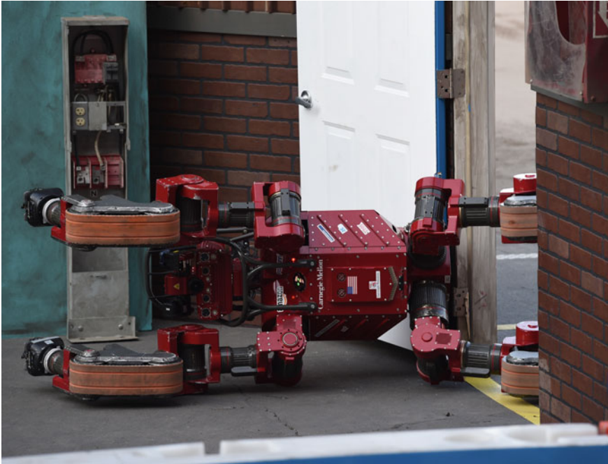
Fig. 21 CHIMP, having fallen through the door opening, during its successful fall recovery maneuver
