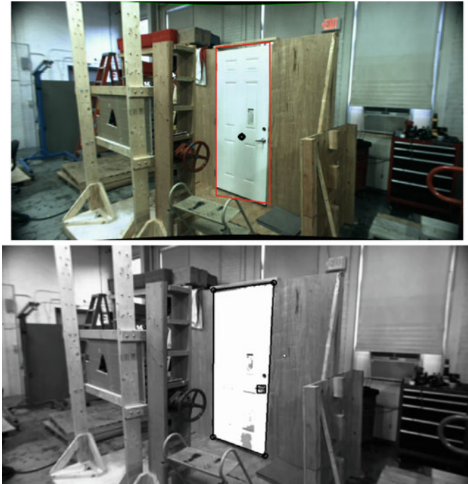
Fig. 13 Detected door and handle in a complex scene
