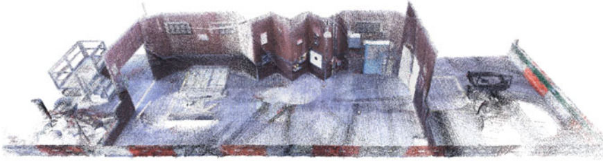
Fig. 14 Colorized LIDAR point cloud resulting from CHIMP’s drift-free pose estimates, captured over the course of an hour navigating the DRC finals course
