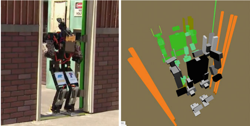
Fig. 23 The operator guides THOR-RD through the doorway with the help of LIDAR feedback over the low bandwidth channel
