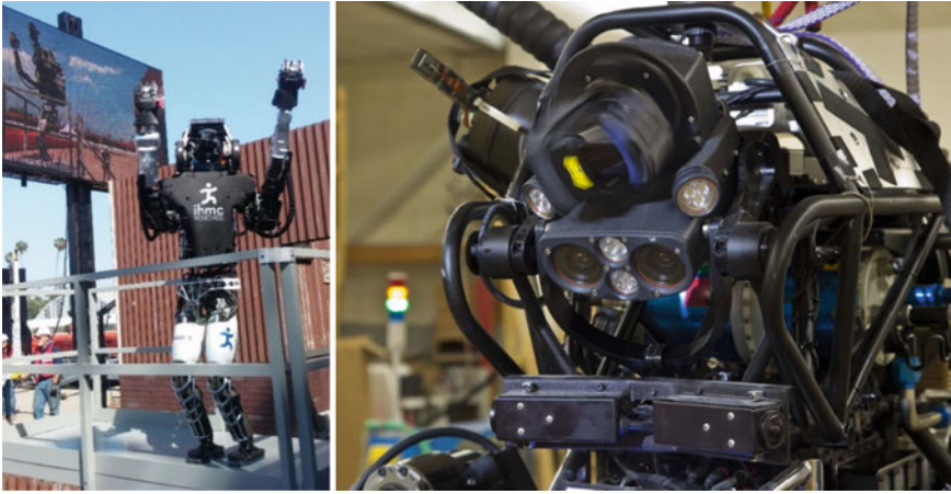
Fig. 2 Atlas robot (left) provided by Boston Dynamics and a close up of the Carnegie Robotics MultiSense-SL head (right)
