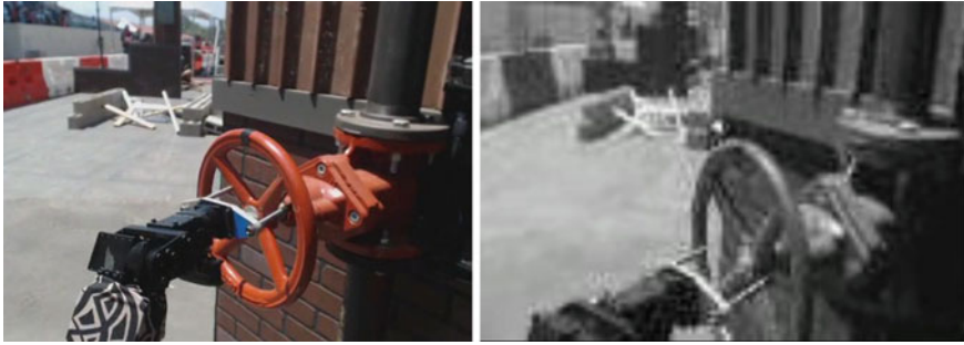
Fig. 24 The high and low bandwidth view during the DRC Finals Valve task: The robust passive hand allows for quick alignment, and the low resolution image feed provides an immediate feedback during operation
