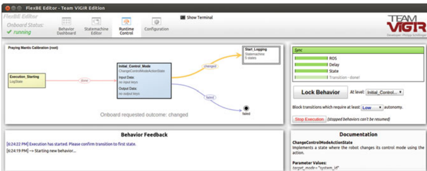
Fig. 10 During system operation, the human operator oversees and directs behavior execution. The active state s (blue) is shown at the center of the Runtime Control view. To its left is the previously executed state. To its right are the possible state outcomes, s_{Oc} = \{\text{changed}, \text{failed}\} , and corresponding transitions, t_{\text{changed}} and t_{\text{failed}} . Once an outcome has been returned by the state, the corresponding transition is highlighted. Here, the behavior is not transitioning autonomously because the current autonomy level ( a_{SM} = \text{Low} ) is not strictly greater than the transition’s autonomy threshold ( a_{\text{changed}} = \text{Low} )
