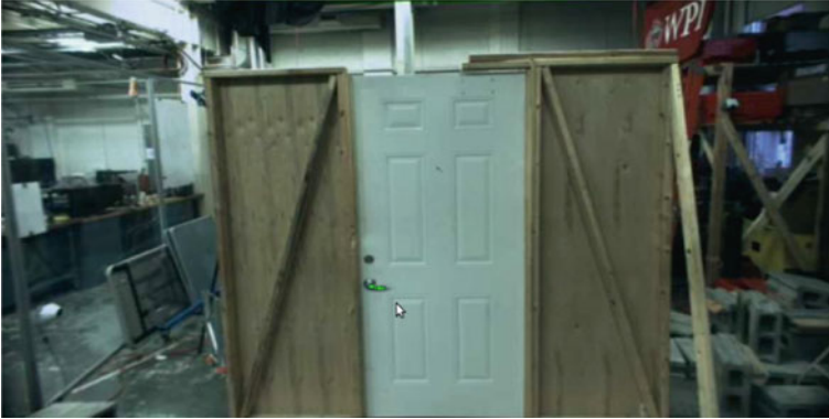
Fig. 15 Operator seed in green color on the handle of the door (near cursor) and the detected door normal
