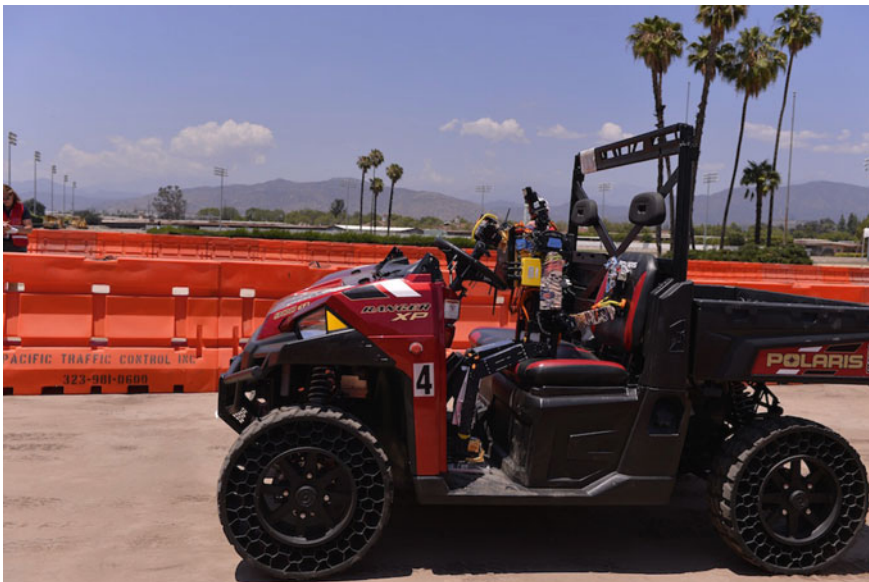
Fig. 22 THOR-RD drives the vehicle with its head rotated 180°. Due to the default birdwalk knee configuration, the robot is mounted backwards in the car
