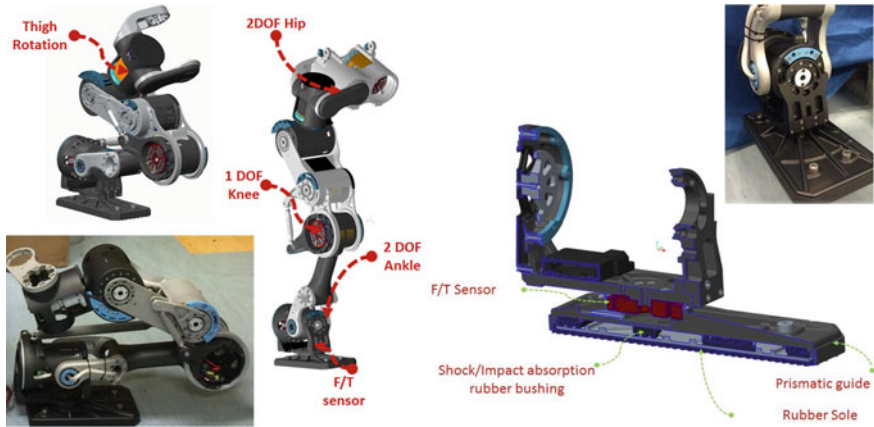
Fig. 9 WALK-MAN leg kinematics and foot design
