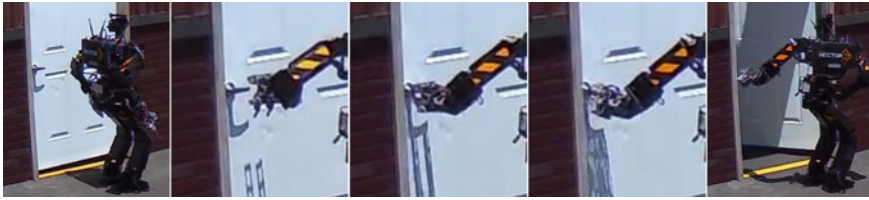
Fig. 21 DRC external footage from the Door task. From left to right: Setup, Pre-grasp, Grasp, Open affordance, Door open
