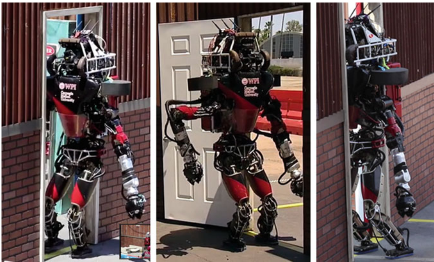
Fig. 1 Detecting Contacts I: Successful sidestepping through the door (left, middle) and the failure in the DRC rehearsal (right) in which the protective cage (black padding) for the head is against the white door frame
