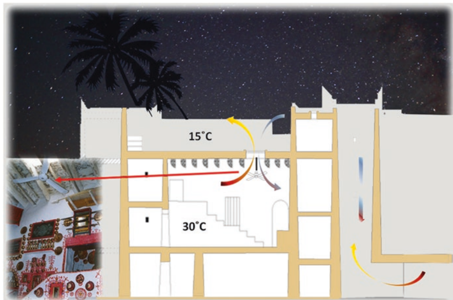
Fig. 7.6 Night ventilation and thermal mass strategies
