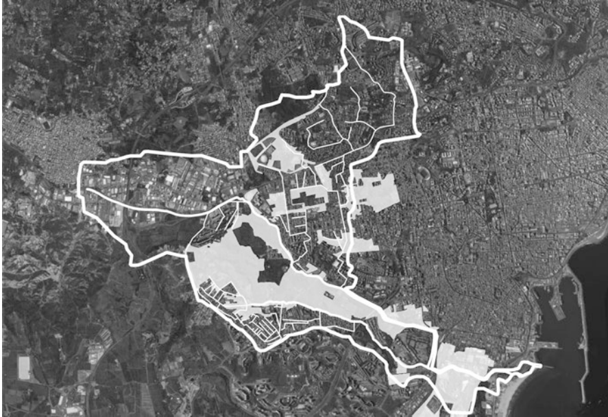
Fig. 6 Modeling of the effects of new urban developments on runoff for a peri-urban basin in Sicily (Italy): in white the areas for the new urban developments for which the release restrictions are defined (Modified from Pappalardo et al. (2016))
