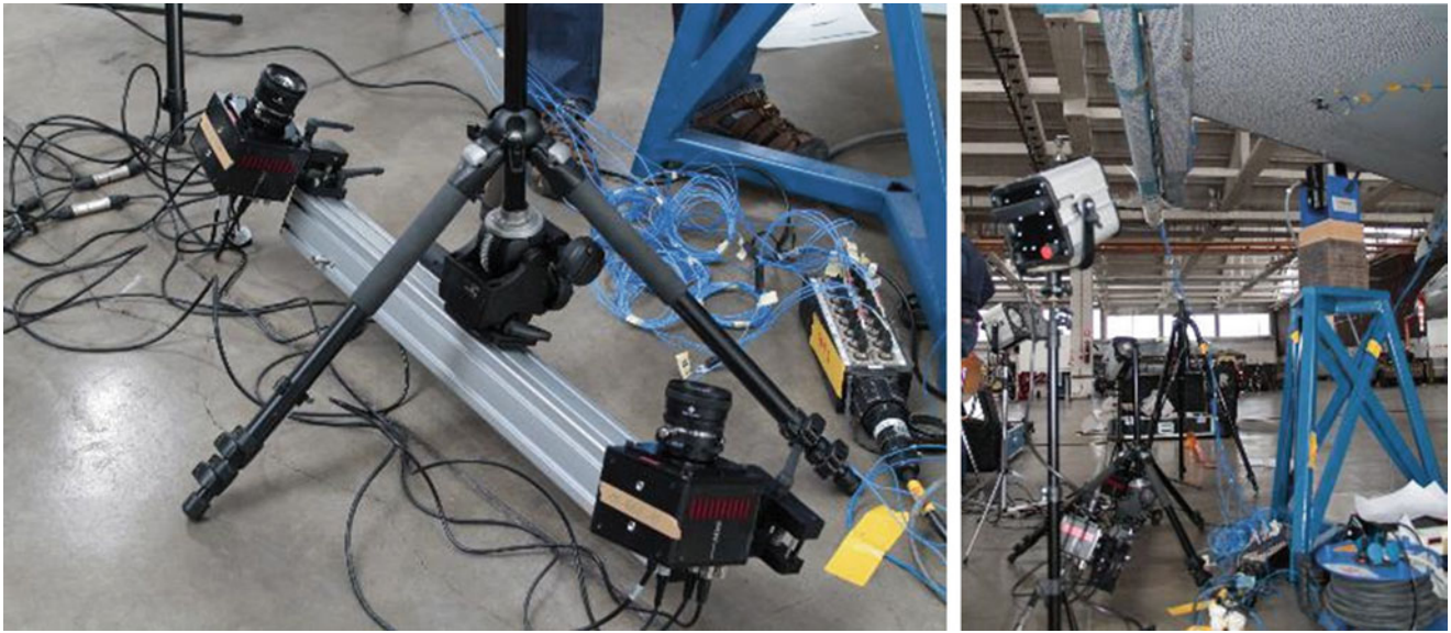
Fig. 5.6 Camera Instrumentation overview with the stereo system on the left and the whole setup with the extra lights on the right
