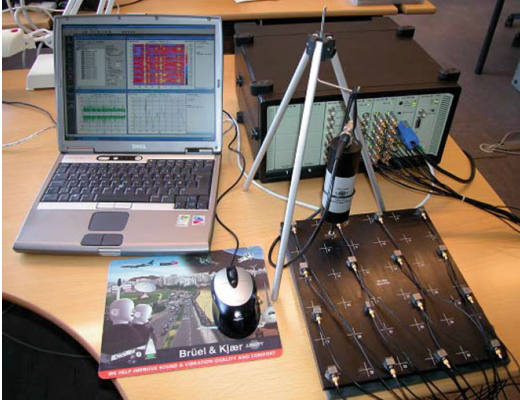
Fig. 2.1 The experimental setup: test plate with 16 acceleration channels, shaker, acquisition system
