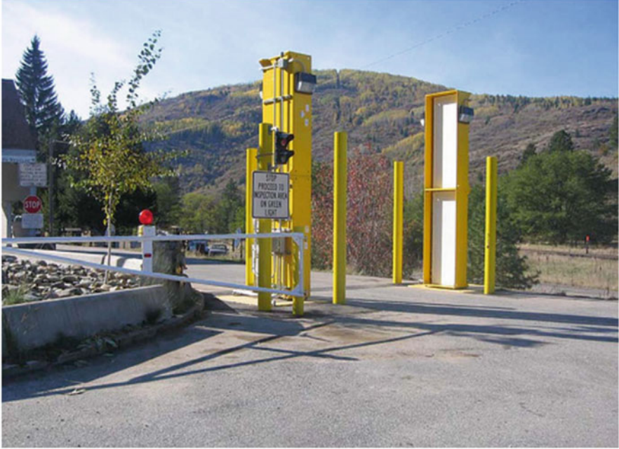
Fig. 3.18 Radiation portal monitor at a test location at Pacific Northwest National Laboratory
