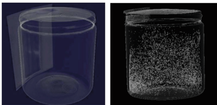
Fig. 6.8 Computed tomography images of an SE detector based on octafluorocyclobutane after photon (1 Gy of 6 MV X rays, left) and neutron irradiation (2.5 mSv of Am-Be, right). Adapted from Ref. [42]
