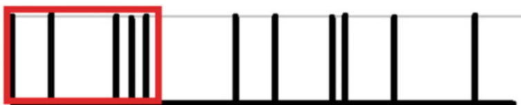
Fig. 6.2 Representation of neutron pulse train where the horizontal axis represents time, each vertical line represents a detected neutron, and the red box is the time window used for creation of the multiplicity distributions
