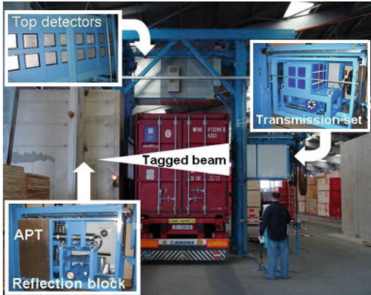
Fig. 9.16 EURITRACK portal during a truck inspection in the seaport of Rijeka, Croatia. Source and detectors are mounted on sliding rails and can be moved up and down to align the tagged neutron beam with the target position. Reproduced from Ref. [18]
