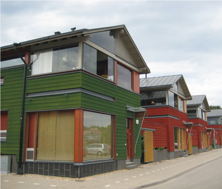
Fig. 5.8 A zero-lot-line design like the one shown here creates more usable space on an overall smaller lot, making it a more sustainable option for new neighbourhood developments
