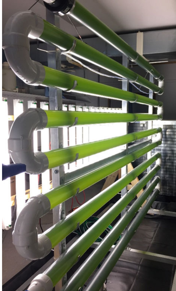
Fig. 4.7 Photobioreactor illuminated (Green Wave Energy, Inc.) by artificial light in pilot-scale laboratory setting at Montana State University, Bozeman MT
