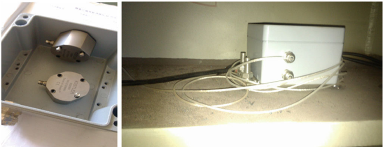
Fig. 11.8 Monitoring measuring chain using MEMS Capacitive sensors and NI PXI-e data acquisition system
