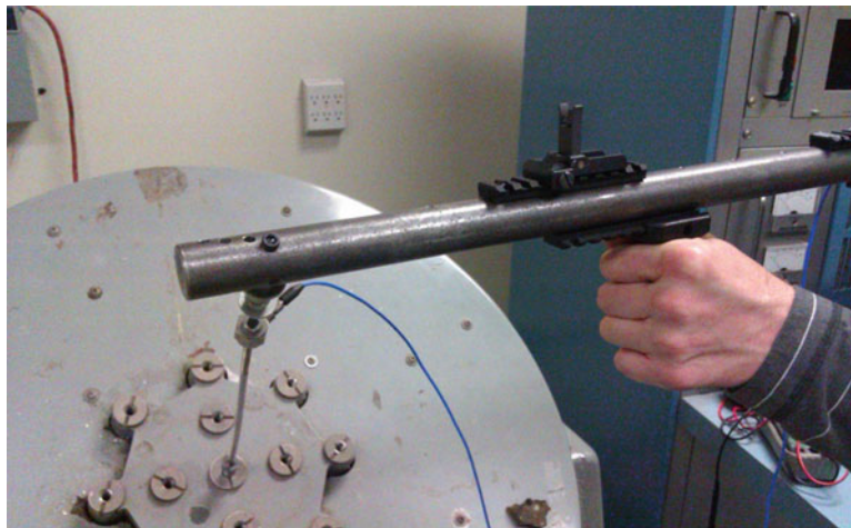
Fig. 1.6 Mock weapon with stinger and shaker setup
