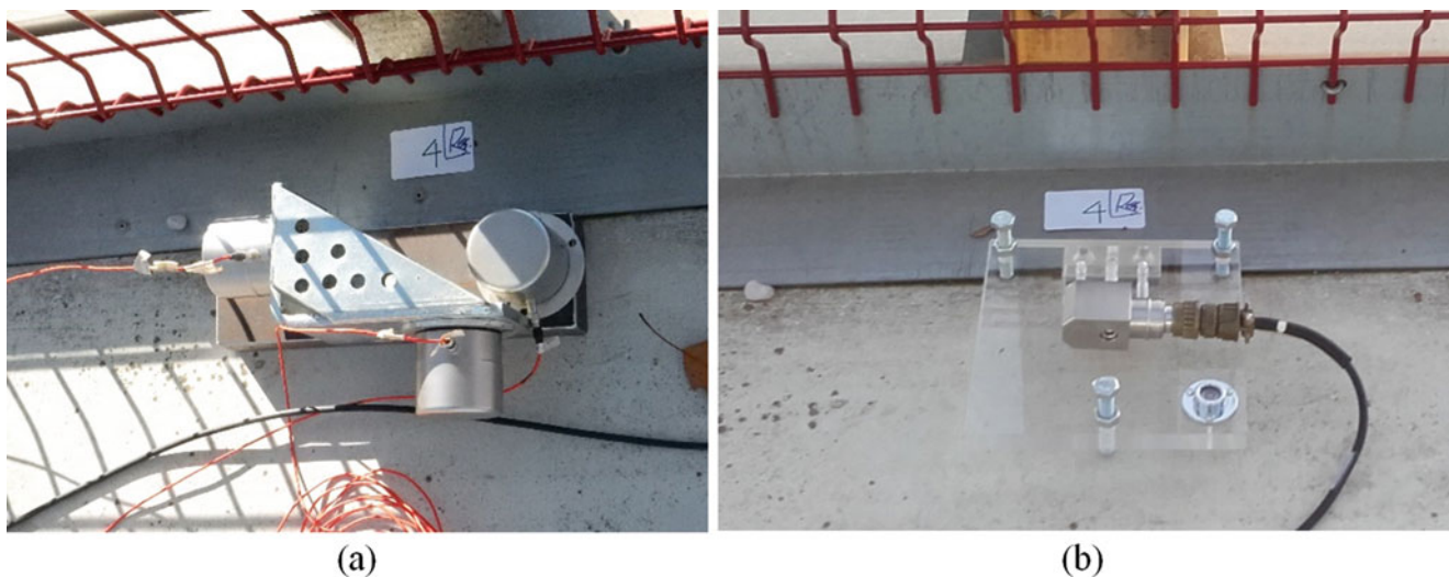
Fig. 22.3 Accelerometers on the deck: (a) Vertical: PCB 393C accelerometer; (b) Lateral: Dytran accelerometer
