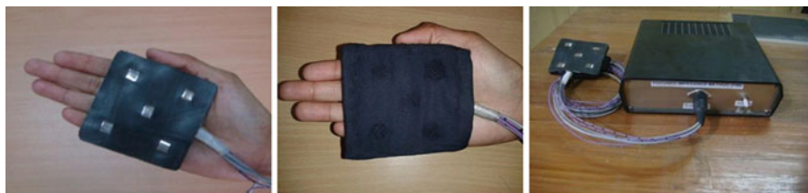
Fig. 9.35 Palm worn four-electrode FIM probe for on a flexible rubber sheet (left), covered by a cotton cloth with wet cotton buttons at the electrodes (middle) for lungs rate measurement on babies using the home made FIM machine (right)
