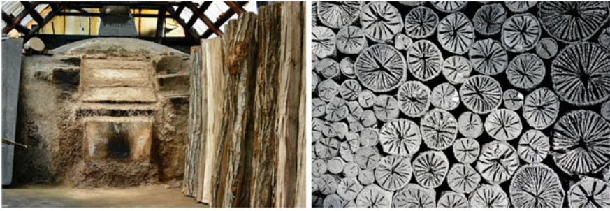
Fig. 8 Oven for producing charcoal and produced charcoal (Noto in Ishikawa Pref., June 29, 2014)
