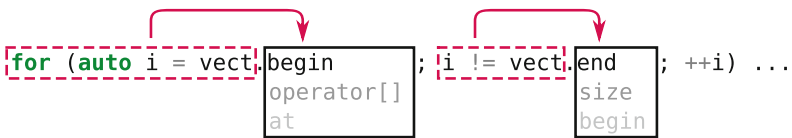
Fig. 1. An example of a context-sensitive completion. The context of a code affects the list of candidates raising only the most probable ones.
