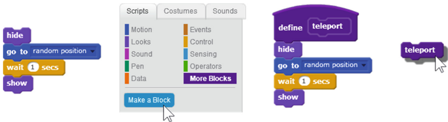
Fig. 1. In Scratch the define hat block is attached to a script, thus defining a new block (Color figure online)
