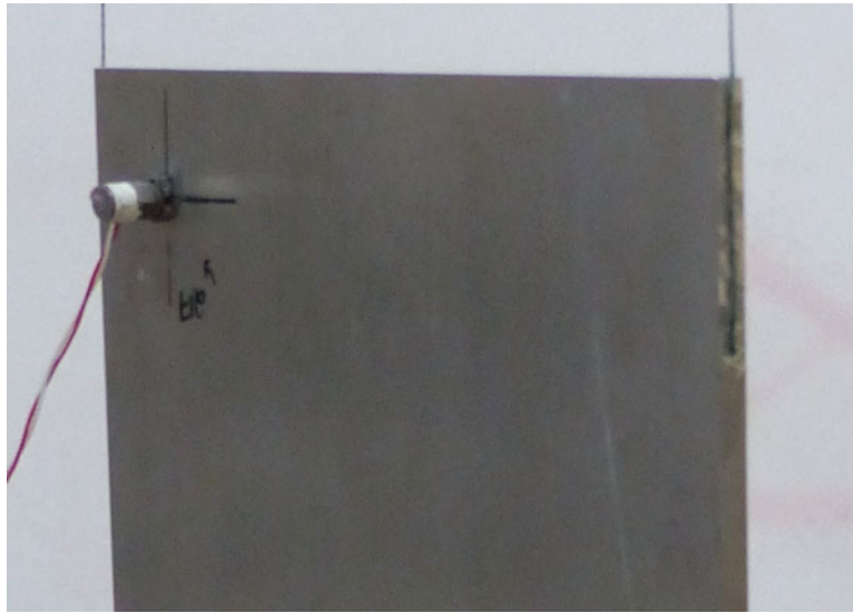
Fig. 23.13 Glued fishing line at the upper corners of the vertically-suspended plates (config. C)
