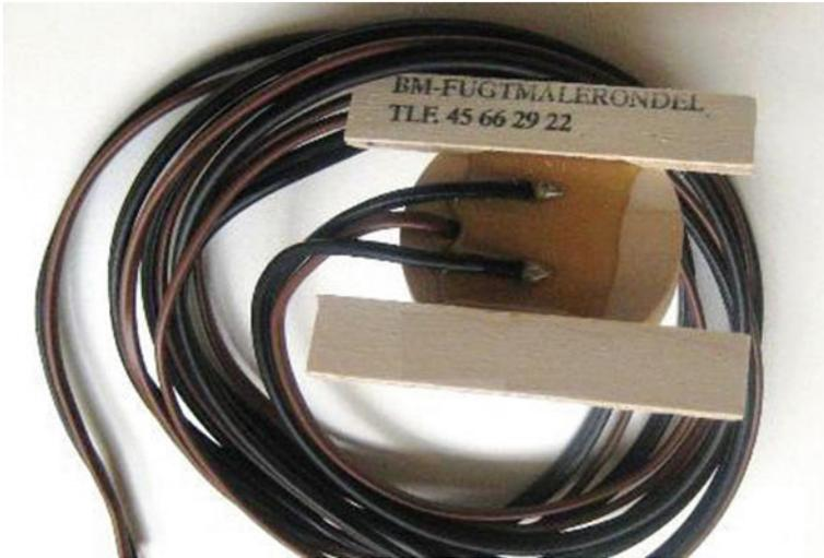
**Fig. 26.10** The wooden rondella for monitoring the moisture variations of its immediate surroundings, BMTInstruments (2016), by monitoring the resistance between the electrodes and the temperature. The electrodes are covered by epoxy coating
