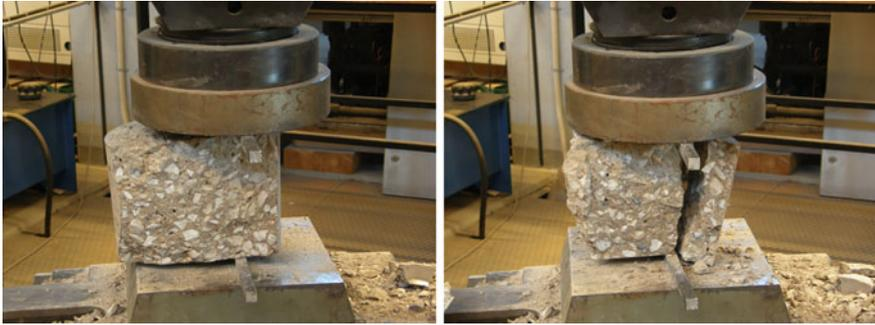
**Fig. 22.1** Splitting a concrete specimen by using rulers and a compressive strength test machine, Johansson (2012)
