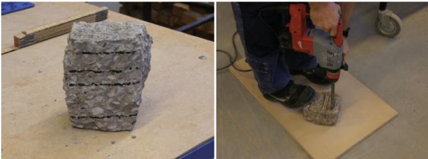
Fig. 22.3 Splitting a large concrete slice into smaller slices and samples with hammer and chisel, Johansson (2012)
