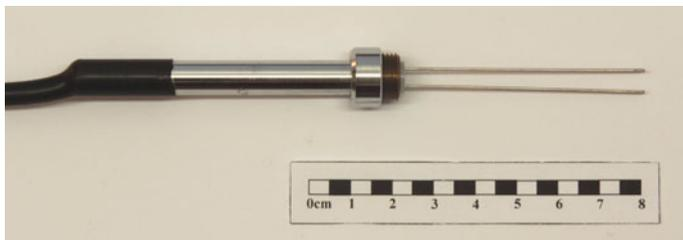
**Fig. 15.2** Two-rod TDR microprobe for laboratory volumetric moisture content measurements in building materials, from Scheffler (2009)
