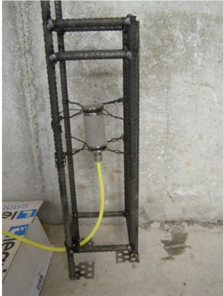
Fig. 23.12 Picture of a “permeability probe” inside a cage
