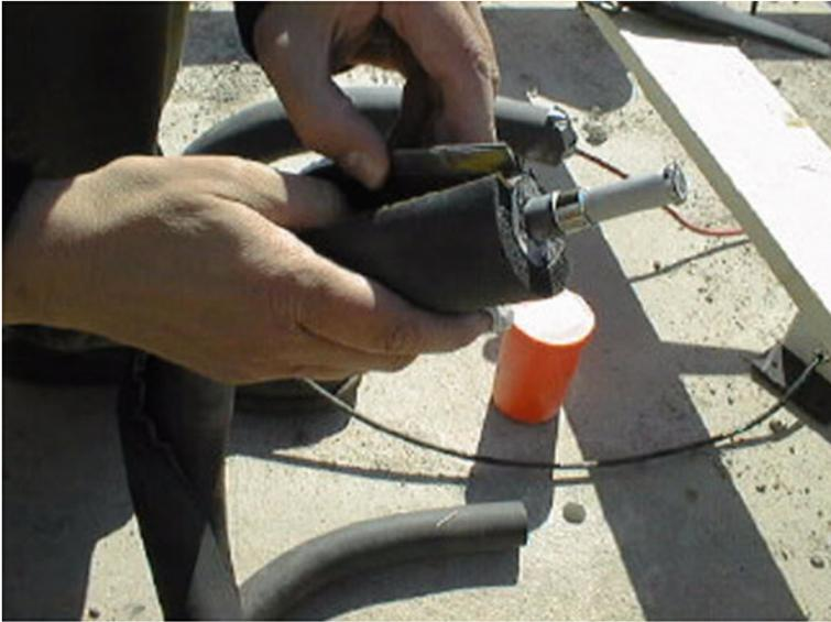
**Fig. 26.5** Heat insulation wrapped around the capacitive RH and temperature probe AHEAD Hygrotemp II. The orange box contains the 'sleeve and cover' insulation where the HMP 44 probe had been put in the drilled whole, Paroll (1997)
