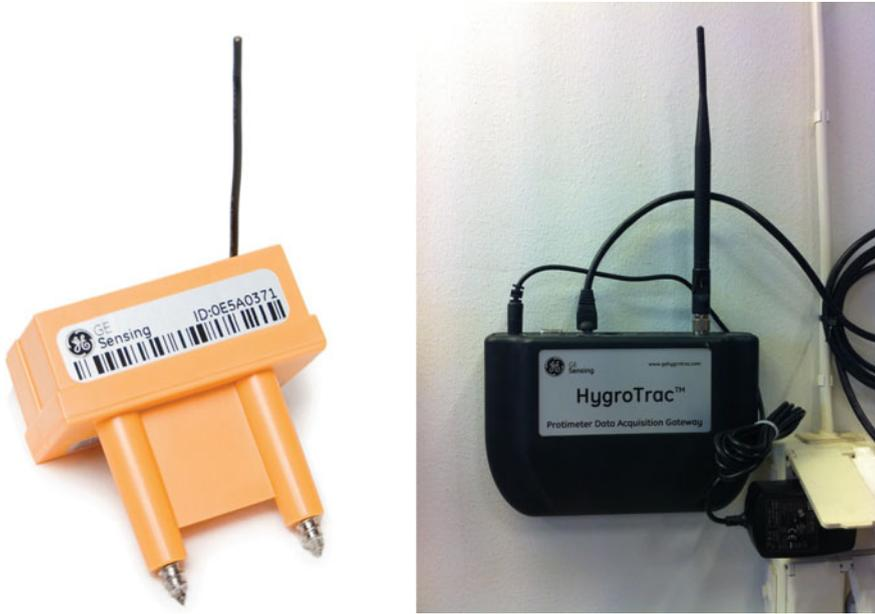
**Fig. 26.11** The wireless sensors (left), Safety express (2016), and the gateway (right) (photo: L-O Nilsson) used by Sandberg et al. (2011)
