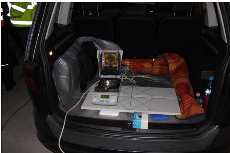
**Fig. 19.17** Determination of reference values using a “moisture balance”
