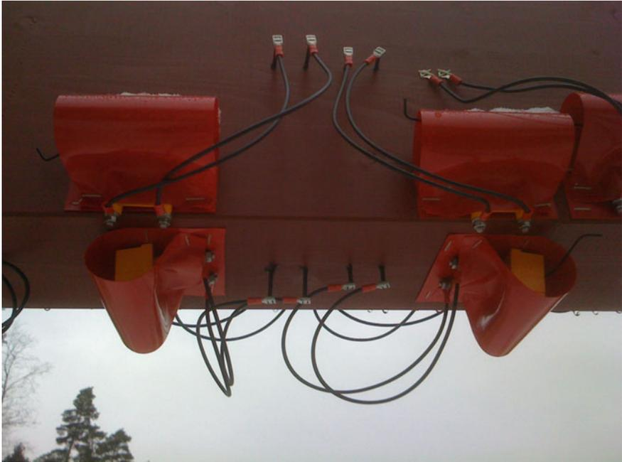
**Fig. 26.12** Five wireless sensors, protected against rain and direct sunlight, each connected to a two-pin sensor or a surface sensor (top right) (photo: L-O Nilsson)
