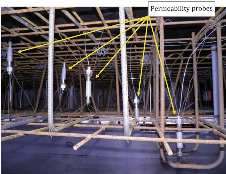
Fig. 23.13 Picture of “permeability probe” disposed in a reinforced concrete wall for moisture profile determination
