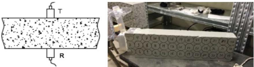
Fig. 24.7 Measurement setup using direct transmission of ultrasound (left) in several positions of an 80 × 20 × 10 cm large, ASR-cracked concrete beam (right) in contact with water at the left end surface, McNair (2015)
