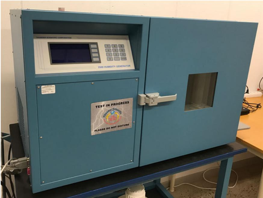
**Fig. 4.3** A two-pressure apparatus by Thunder Scientific Corporation at the Laboratory of Building Materials at Lund University (photo L.-O. Nilsson)
