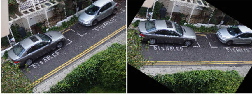
Fig. 5.9 Rotating a camera image. a Source image. b Rotated so that the double yellow line is horizontal
