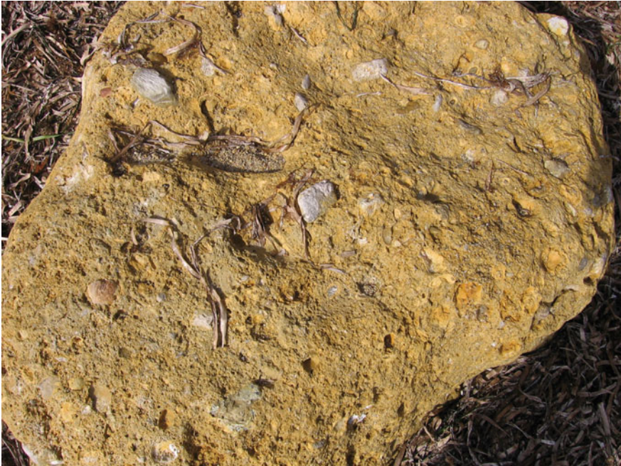
Fig. 2.104 Calcirudites and coarse calcarenites of the Marsala synthem. The breccia displays elements deriving from the dismantling of the Mesozoic carbonate substrate; the rock is well cemented and rich in shell fragments, as molluscs, crinoids, anellids, corals (Punta Raisi, Palermo)
