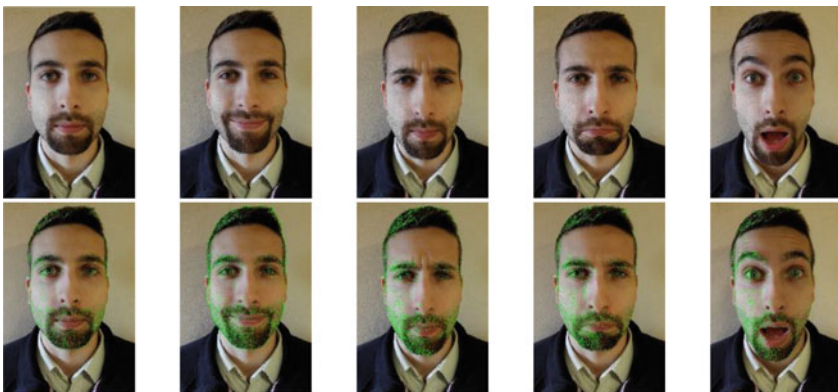
Fig. 2.3 SIFT features: the first five images (first row) show some well-known facial expressions: neutral, smiling, altered, doubtful, surprised. The other images (second row) show the extraction of the SIFT features on them
