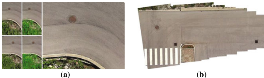
Fig. 2.5 SURF algorithm: a Running example of a mosaic composed by 2 frames. The first 2 frames (first column) are the original ones acquired by the UAV, the other 2 frames (second column) are the same frames in which the SURF features are extracted, the comprehensive view (third column) is the mosaic obtained by the stitching (based on the features), b example of mosaic composed by 9 frames
