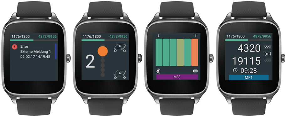
Fig. 6. Different monitoring and control services on the smartwatch
