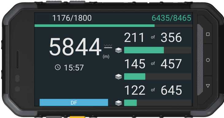
Fig. 3. Remaining time of current job and stack size modules on smartphone
