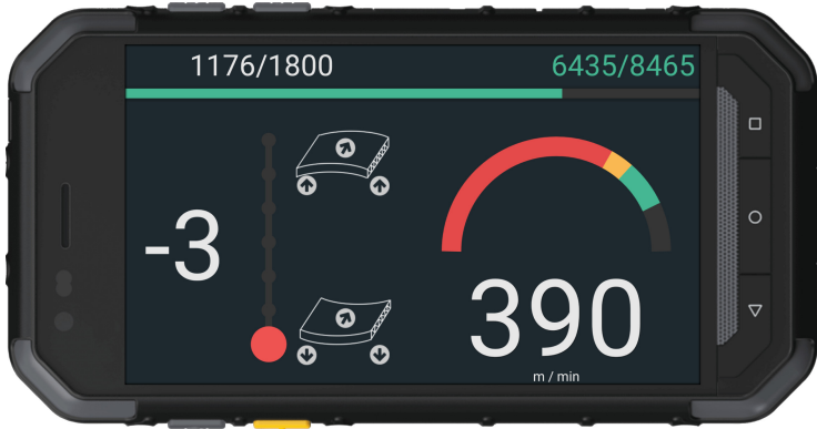
Fig. 4. Warp control service and current production speed on smartphone
