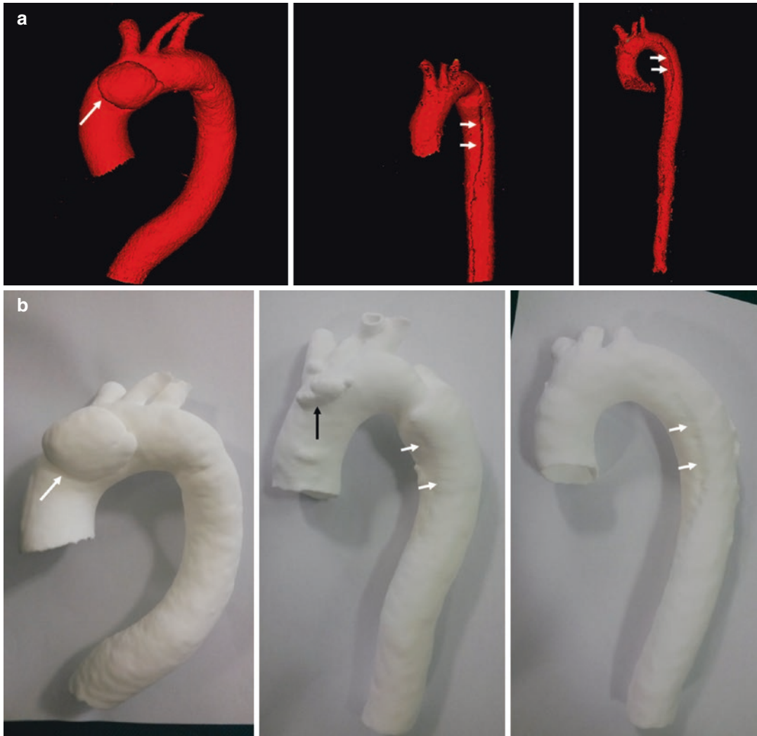
Fig. 38.4 3D printed patient-specific models of aortic aneurysm and aortic dissection. (a): 3D segmented reconstructions of aortic aneurysm (first image), and Stanford type B aortic dissection (second and third images) based on CT angiographic images. (b): 3D printed models of aortic aneurysm and aortic dissection. White long arrow
