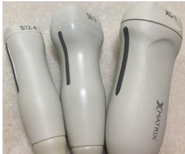
Fig. 17.1 Ultrasonic probes used for a focused cardiovascular ultrasound (FOCUS) examination. The black line on each probe helps identify the image orientation on the screen. The number is the frequency of the transducer in megahertz, i.e., S12-4 is 12–14 megahertz. A smaller probe with higher frequency has a smaller footprint, which is useful in infants
