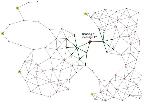
**Fig. 5.** The reference node asks for local minima nodes (flooding messages).
