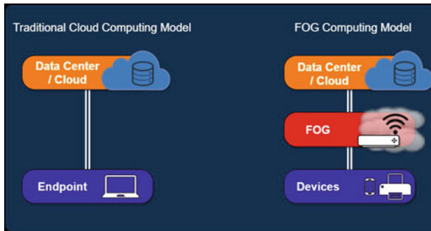
Fig. 12.2 Traditional cloud computing model versus Fog computing model
