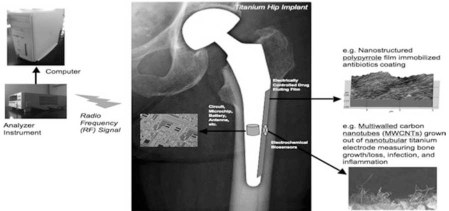
Fig. 7 Electrochemical detection of bacteria, inflammation, or bone growth surrounding a hip implant. The intelligent hip implant utilizes carbon nanotubes grown out of anodized tubular titanium to detect what type of cell attached and tissue is forming. Further, it sends such information to a hand-held device and can be remotely activated to release bone growth factors, anti-inflammatory agents, and/or antibiotics to ensure implant success
