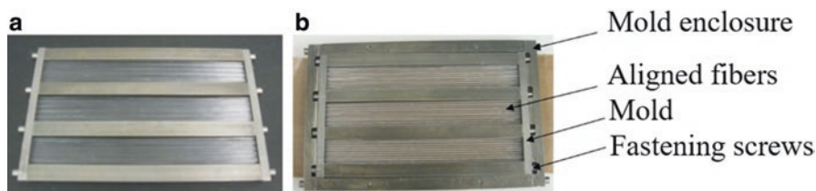
Fig. 2 Setup of the fiber arrangement in the mold (a) fiber aligned in the mold and (b) mold seated in its enclosure to retain the polymer
