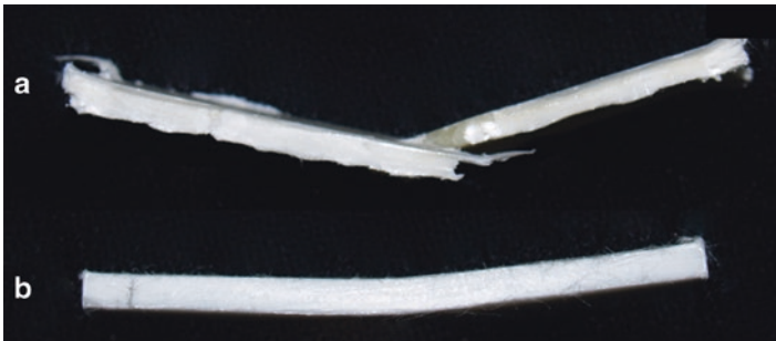
Fig. 10 Composite bars after 3-point bending testing made by Heimbach et al. [81] containing PLLA, HA, and PCL. (a) A composite containing 23 vol% HA that suffered from brittle failure, and (b) shows the ideal composite composition from this study containing 15 vol% HA. Note the toughness of the composite in (b), showing no brittle failure and good shape retention. B. Heimbach et al., J Biomed Mater Res Part B. 2016 , 105B, 1968
