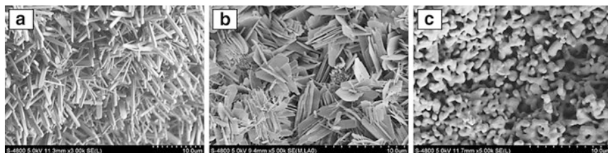
Fig. 4 Representative SEM images of hydroxyapatite ceramics synthesized using hydrothermal method: (a) one-dimensional rods; (b) two-dimensional plates; (c) short-rods/spherical shape
