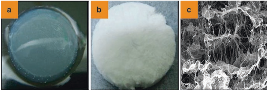
Fig. 4 Porous collagen scaffolds fabricated via freeze-drying: Optical image of collagen gel scaffold (a) before and (b) after freeze-drying. (c) SEM image of a freeze-dried collagen scaffold. Figures reproduced with permissions [88] © 2015 IOP Publishing Ltd
