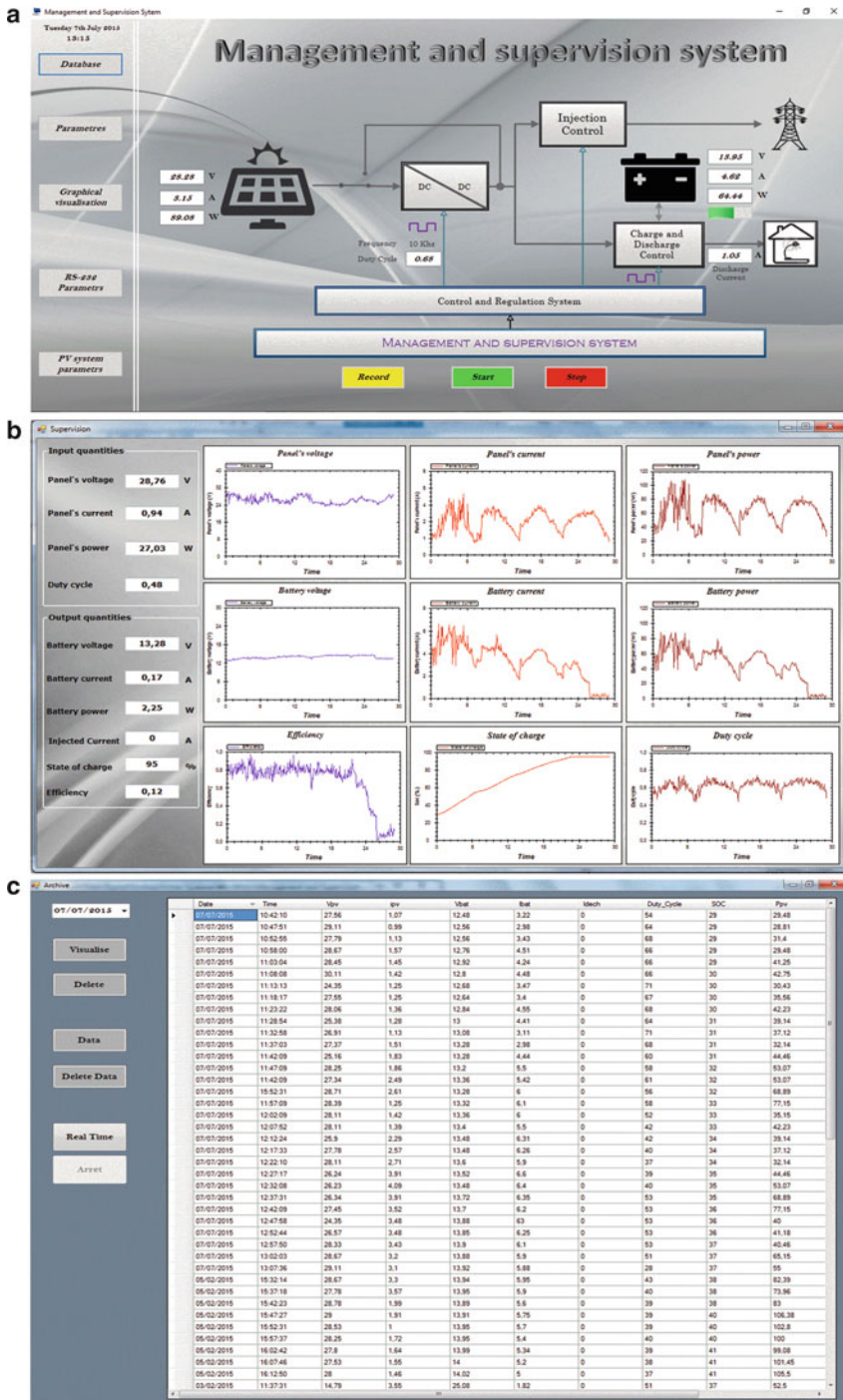
Fig. 19 Management and supervision software during the operation of the PV system. (a) Main software window. (b) Graphical plots of electrical quantities. (c) Database of electrical quantities
