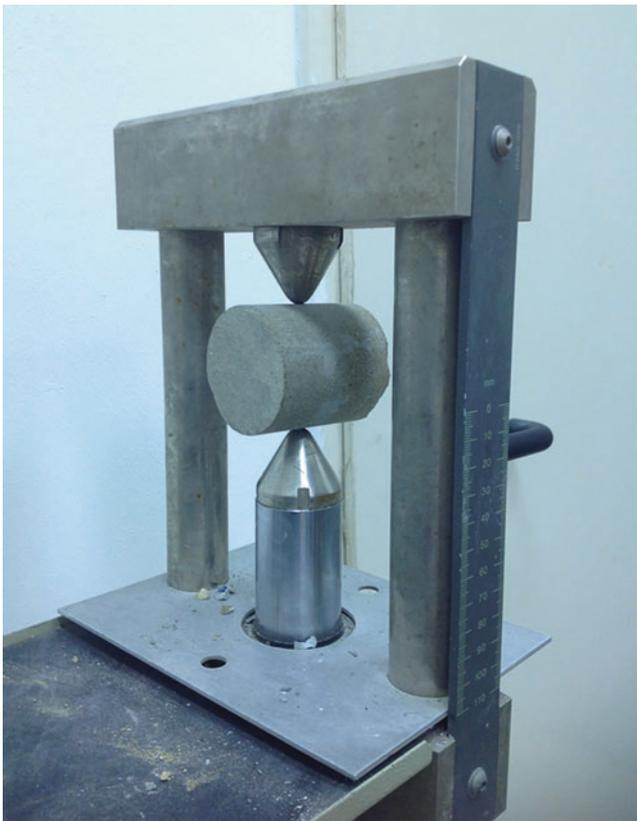
**Rock Laboratory Tests, Fig. 4** Point load strength test (diametral test)
