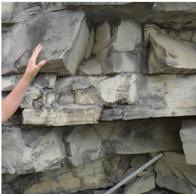
**Rock Mechanics, Fig. 1** Silty limestone (micrite) rock mass exposed along a highway road cut, including intact rock blocks separated by discontinuities (subhorizontal bedding planes, two steeply dipping joint sets, and a few additional randomly oriented joints) (Photo by D. Jean Hutchinson)
