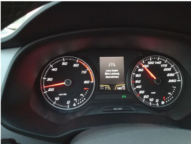
Fig. 11.6 Lane keeping assistant (LKA) ADAS function in a Seat Leon; driver must take up control again
