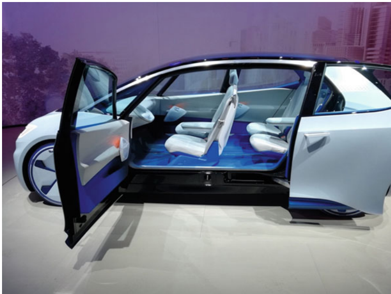
Fig. 11.22 If the car drives autonomously, the steering wheel is retracted and does not occupy space in the interior design
