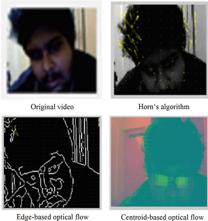
Fig. 11.13 Detection of moving objects and motion (see Bhattacharjee 2013)
