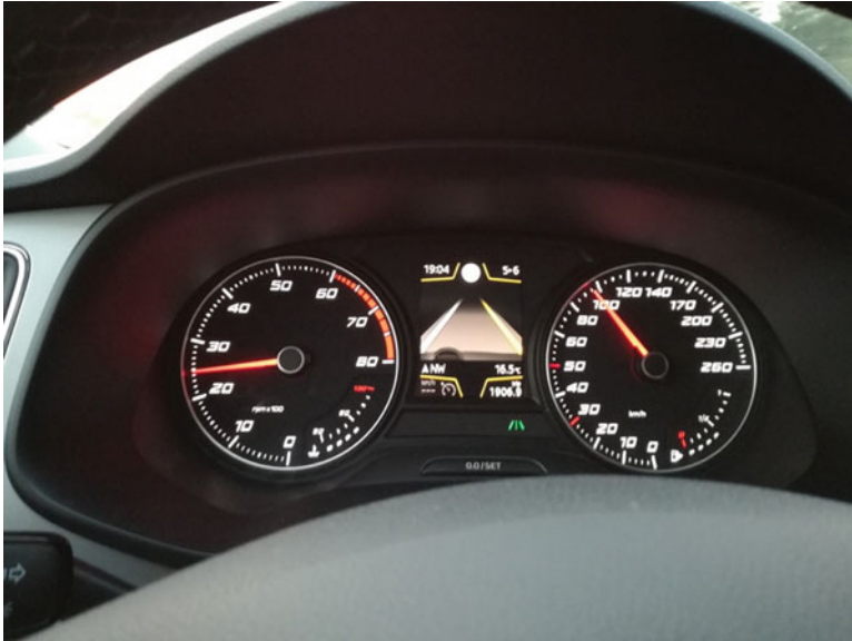
Fig. 11.5 Lane keeping assistant (LKA) ADAS function in a Seat Leon
