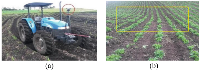
Fig. 2. Acquisition process: (a) Vision system installed on tractor; (b) Location of the region of interest (ROI) into an image
