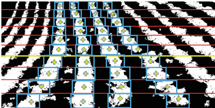
Fig. 10. Location of micro-ROIs (blue rectangles) along crop rows that cross the top and bottom edges of the ROI.
