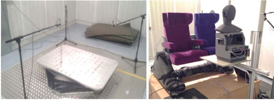
Fig. 1 Left, Multi-axial low noise vibration table in a semi-anechoic room. Right, Seats installed in the vibration table together with a binaural recording system
