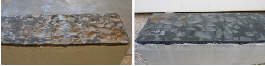
Fig. 12 The elastic and plastic material properties of under-sleeper pads combined forecasted and desired ballast impressions immediately after removal (left) and three weeks later—complete restoration (right)
