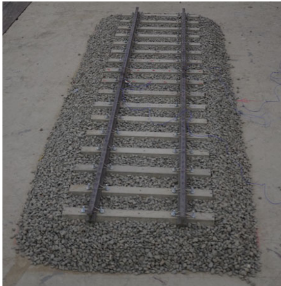
Fig. 5 Experimental set up for the 1:5 scale whole track embedded in ballast
