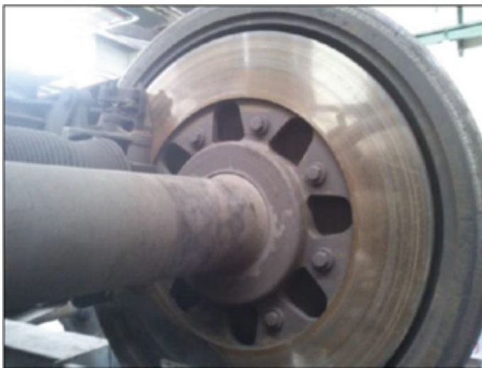
Fig. 1 Disk brakes, in this case a wheel disk brake
