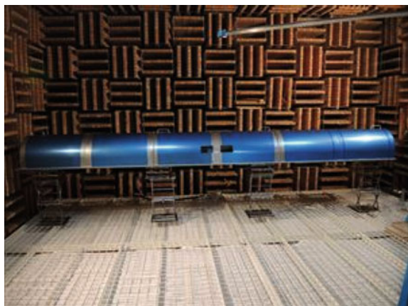
Fig. 6 Model of tunnel hood
