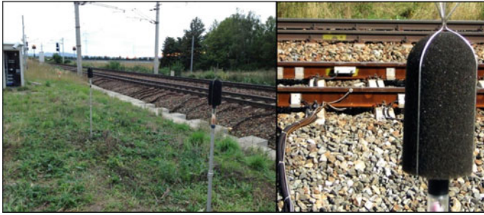
Fig. 1 Noise monitoring station at Deutsch-Wagram in Austria
