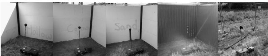
Fig. 2 Unattended noise monitoring set-up
