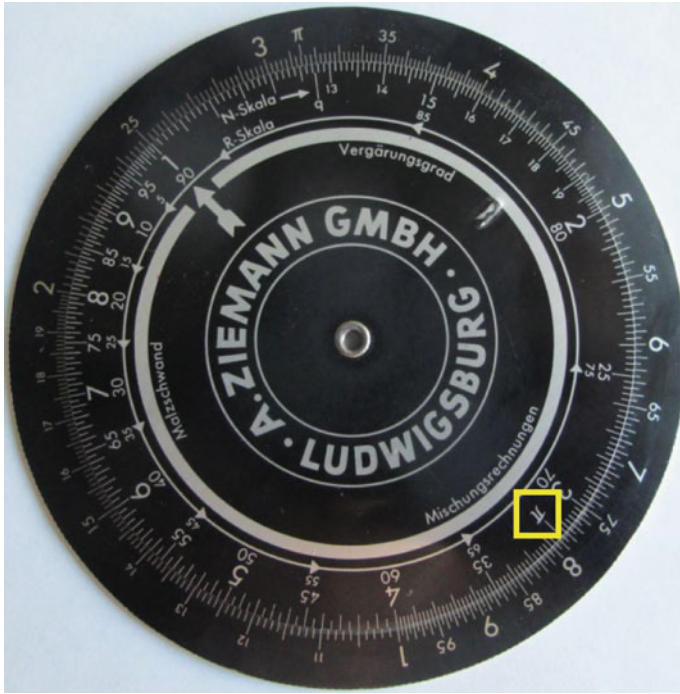
Fig. 1 A circular slide rule from ca. 1960 Author’s photo
