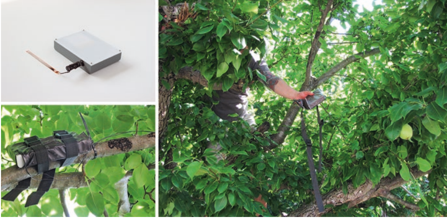
Fig. 9.6 Fruit sensor, sensor installed on tree, being taken down
