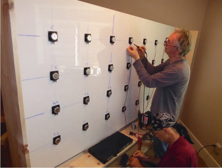
Fig. 13.1 The Pixelphonic prototype. 8' × 4' 3 mm Alupanel screen for projection-based display, utilizing an 8 × 4 2D array of audio exciters to vibrate the screen from its backside (author's image)
