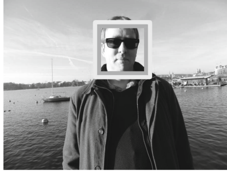
Fig. 6. Face detection and marking in photos using OpenCV with Python 2.7
