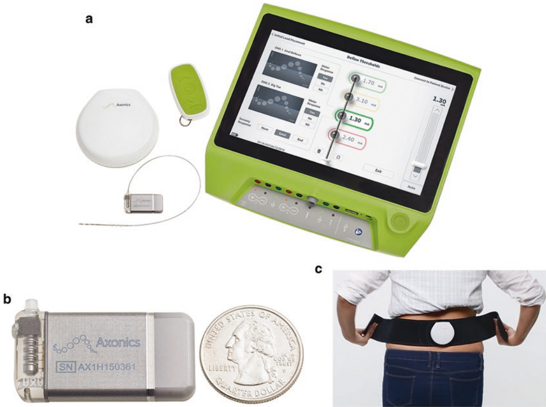
Fig. 13.3 The Axonics sacral neuromodulation (a) full system, (b) implantable pulse generator with rechargeable battery, and (c) wearable flexible belt with recharging
