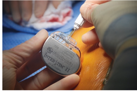
Fig. 3.16 The Model 3058 pulse generator connects directly to the free end of the neurostimulator lead by tightening the single set screw with the supplied torque wrench
