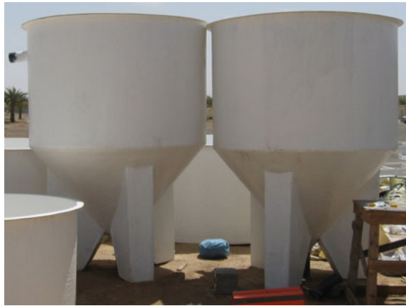
Fig. 7.13 Clarifiers with 60° conical bottoms
