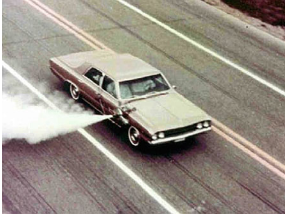
Fig. 6.67 Lateral force applied by means of a rocket (General Motors Corporation, circa 1960)
