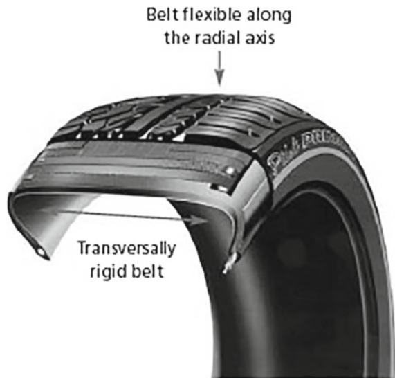
Fig. 2.3 Structure of a radial tire [11]
