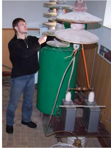
Fig. 1. Insulator testing unit
