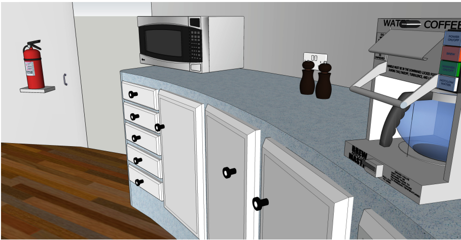
Fig. 2. The designs considered all the necessary details to produce final real model. For example, the handle to assist the person in wheelchair, the fire extinguisher for safety, the sockets, coffee maker, and other details.
