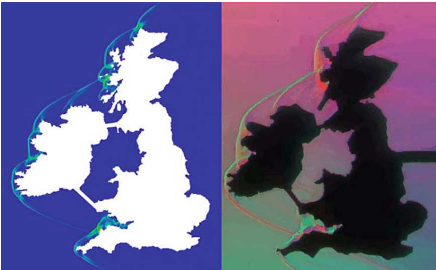
Fig. 5 Qualitative contours of density gradient. Left: results from rhoCentralFoam . Right: Experimental colour schlieren results
