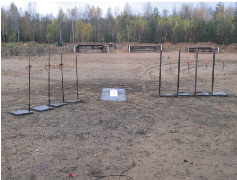
Fig. 5 Two rows, each composed of four pressure transducers and situated at the plane angle to each other, installed near the TNT charge at the field test [11]
