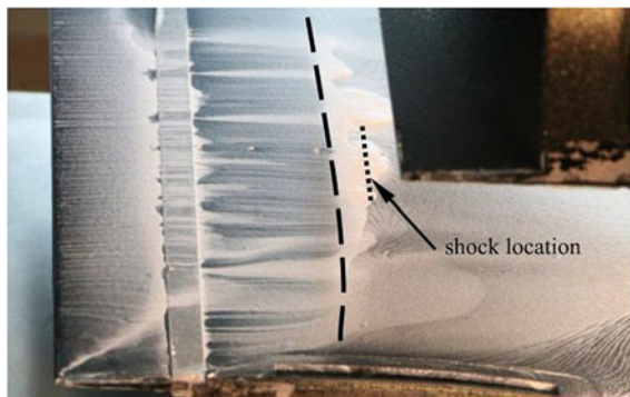
Fig. 9 Oil visualisation for turbulent interaction, step at X/C = 0.16
