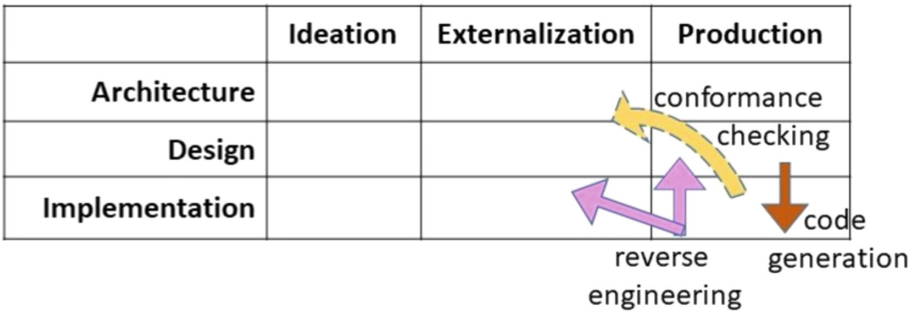
Fig. 11. UML tools across design stages
