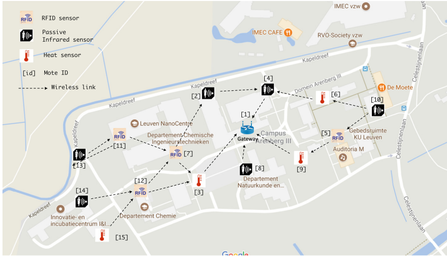
Fig. 6. Configuration area security surveillance application
