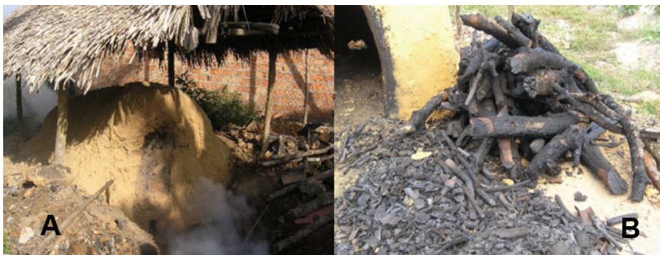
Fig. 29.6 The manufacturing process of charcoal using mangrove wood
